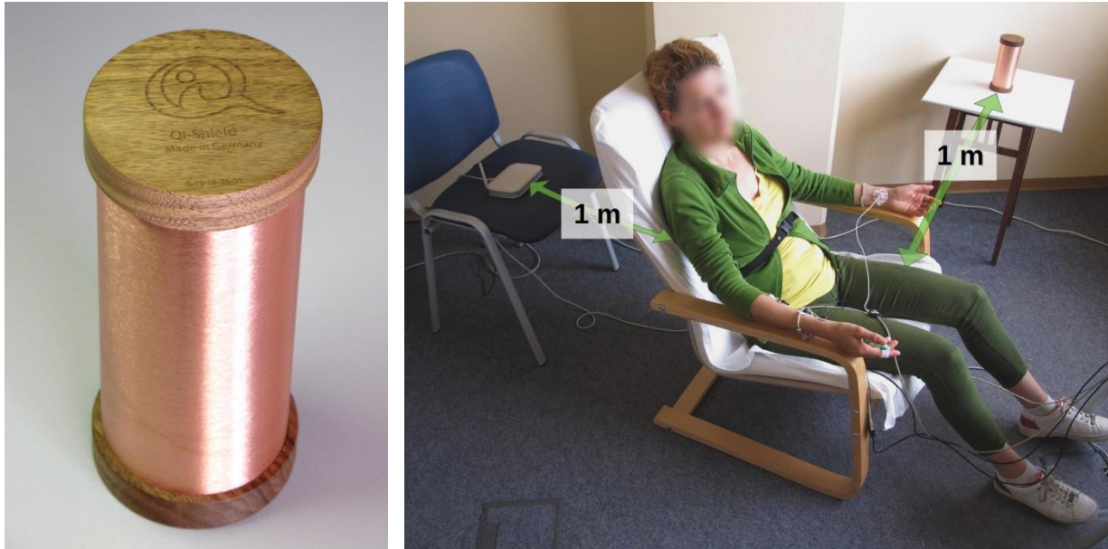
Figure 1: (a) Specimen of the Qi-Shield device used for testing (left). (b) During the measurements volunteers sat in a comfortable wooden chair with electrodes attached to both hands and Qi-Shield and Wi-Fi router placed 1 m away from them (right).
