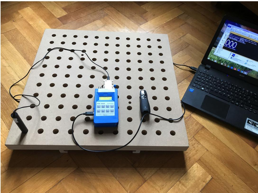
**Fig. 3:** Magnetic field measuring apparatus with wooden measurement board and measuring grid, probe (black, left), meter (blue, center), presenter for taking measurement values (black, to the right in the measuring field) and measuring computer for data storage (to the right in the photograph)
